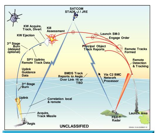
Firing Ship Engages Threat Using Remote Track Data
